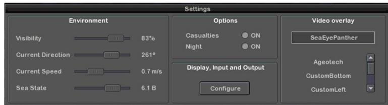
The Video Overlay panel allows you to choose from a list of available configurations. This way ROVsim<sup>2</sup> Pro may be used to simulate a number of manufacturers' systems. Additional overlay configurations as well as custom configurations may be added.
